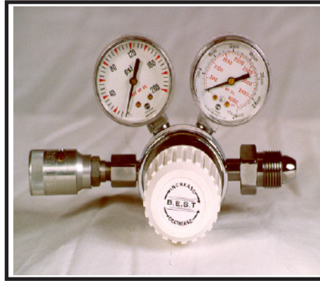
Adjustable, 0-200 PSI, Diaphragm 2" Gauges & Schrader Female
